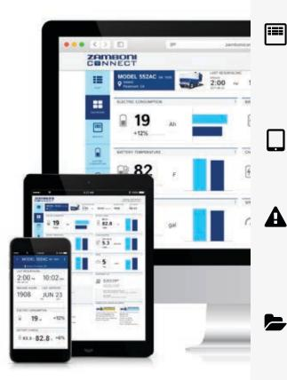
WiFi Requirements: WiFi router with a minimum signal strength of -70 dBm and is compliant with IEEE 802.11 b/g/n. A dedicated router for Zamboni Connect<sup>®</sup> system is recommended. Best location for router installation is in machine storage room, or line of sight to machine storage room or ice pad.
